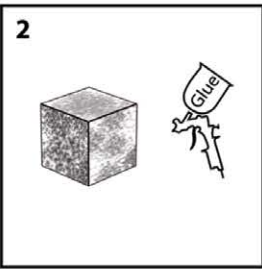
2-Apply glue back of the panel
