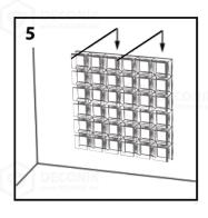
5-Push the panel to contact glue with desired location
