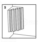
5-Push the panel to contact glue with desired location
